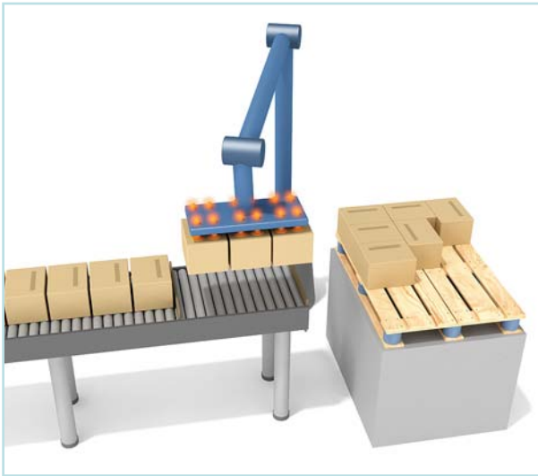
MultiPick/SinglePlace with vacuum gripper
